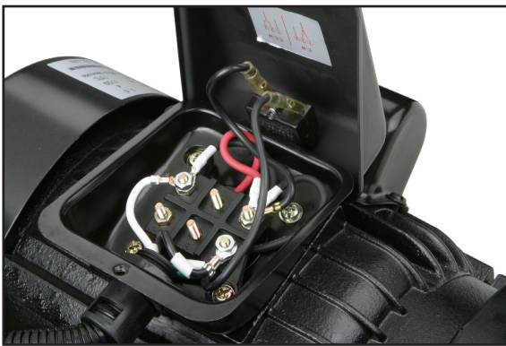
Figure 48. Junction box (M1).
